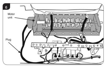
6.1 The motor & effects unit is attached by 4 x screws located at the rear of the appliance. It may be necessary to move the appliance from its location to gain access to the rear of the appliance. Remove the 4 screws on the lower rear casing.
