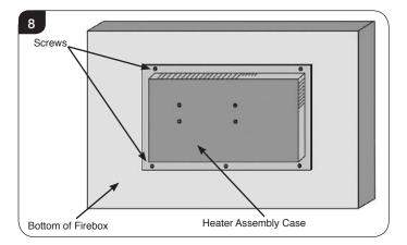
9.3 Remove the 4 screws from the front of the heater casing, see Diagram 9 to free the heater assembly.
