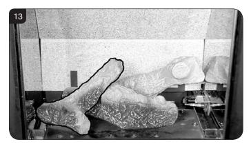
7.5 Place the small Ember at the front left of the firebox, against the rear of the log support broket to obscure the reflection of the burner screw.
