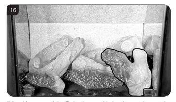
7.8 Use some of the Embaglow provided and cover the ports in the burner tray with a liberal amount of fibres. Use a small piece in front of the log on the left hand side and a long strip in front of log B, see Diagram 17.
