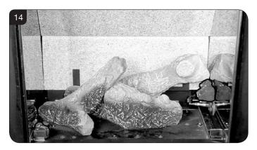
7.6 Log C rests on the cutout on Log E and is pushed up to the side and rear of the firebox, see Diagram 15.
