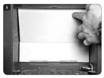
4.6 The lower rear liner does not need to be removed from the bracket in order to access the burner tray for maintenance, but can be lifted off in order to clean or replace, see Diagram 6.
