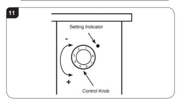
5.10 The exact setting of the thermostat and the manual Air Controls may need slight adjustment by trial and error to suit requirements.
