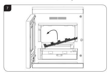
6.9 Lift the multi-fuel frame and rotate to remove from the firebox.
