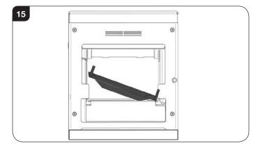
6.4 Place tray flat on the fixings on the firebed, see Diagram 16.
