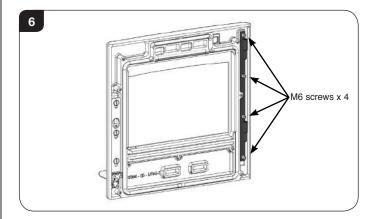
The hinge plate assembly is slotted so it can be moved up, down and sideways by approximately 3mm to adjust the position of the door in relation to the appliance.
