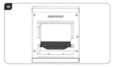
6.5 Fit the plug supplied into the hole where the riddling mechanism is normally located and secure with bolt and clamp (also supplied), see Diagram 17.
