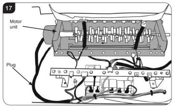
9.1 The motor & effects unit is attached by 4 x screws located at the rear of the appliance. Remove the 4 screws on the lower rear casing.
