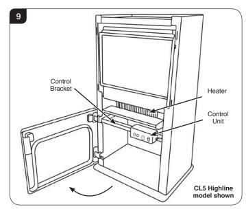
4.15 Remove the 2 screws securing the control unit to the underside of the control bracket, see Diagram 10.
