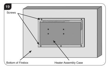
12.4 Remove the 4 x screws from the front of the heater casing, see Diagram 20, to free the heater assembly.
