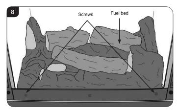
5.1 Lift the fuel bed carefully out through the front of the appliance.
