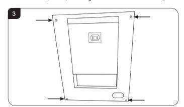
4.3 Remove the main door casting to gain complete access to the engine and the viewing aperture by lifting the hooks clear of the slots on the front of the appliance, see Diagram 4.
