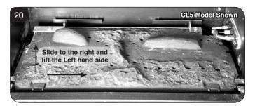
5.4 Slide the burner back to the left and out of its location. IMPORTANT: Take care when removing the burner not to damage the ceramic pad with the pilot unit attached.
