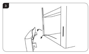
5.3 Remove the frame to gain complete access to the control valve and the viewing aperture by lifting the hooks clear of the slots on the front of the appliance, see Diagram 4.
