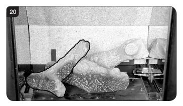
9.5 Place the small Ember at the front left of the firebox, against the rear of the log support bracket to obscure the reflection of the burner screw.
