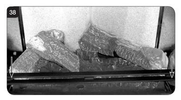
9.23 Place Log A across Log C. There is a hole on the underside of Log A which fits over the raised stud on Log C to secure in place. The small cut out on the left side of the log rests onto the log guard, see Diagram 39.
