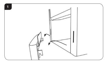
3.2 Remove the frame to gain complete access to the control valve and the viewing aperture by lifting the hooks clear of the slots on the front of the appliance, see Diagram 2.
