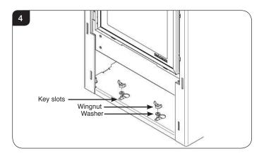
3.7 Place the two large washers over the studs and fix with two wingnuts, see Diagram 4.
