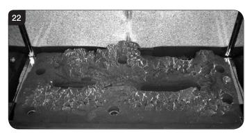
7.18 There are 3 embers. Place 2 embers in the back corners of the burner, resting in the cut outs, see Diagram 23. Place the last ember loosely at the front of the fuel bed to cover the hole in the centre.
