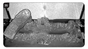
9.20 Place Log B on top of Log D. There is a hole on the underside of Log B which fits over the raised stud on Log D to secure in place. The right hand side of the log rests in the groove in the burner, see Diagram 36.
