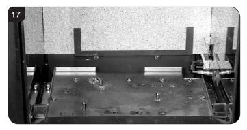
9.2 Place Log A on the higher rear bracket and push up against the back panel, see Diagram 18.
