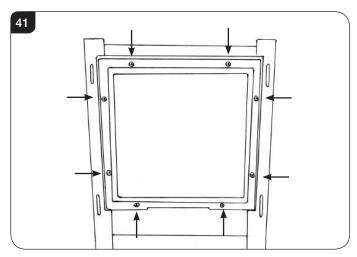
10.2 Replace ALL of the glass frame securing screws ensuring that a screw is present in all fixing slots.
