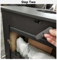
Notice that one side of the slider has a stopper that protrudes and a hole in the centre for the air control.
