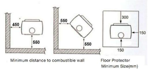
It is recommended that the stove be installed at least 500 mm from combustible materials. However, any household furnishings should be at least 1000mm away as they could be adversely affected by heat.
