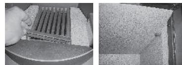
Top baffle brick 11 (smallest straight edge resting on top edge of rear brick) fitted and supported with two side pins.
