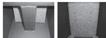
Rear brick 8 fitted in line with tertiary air holes.
