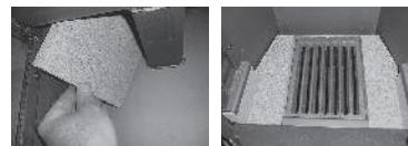
Base bricks, grate, spacer and small side bricks.
