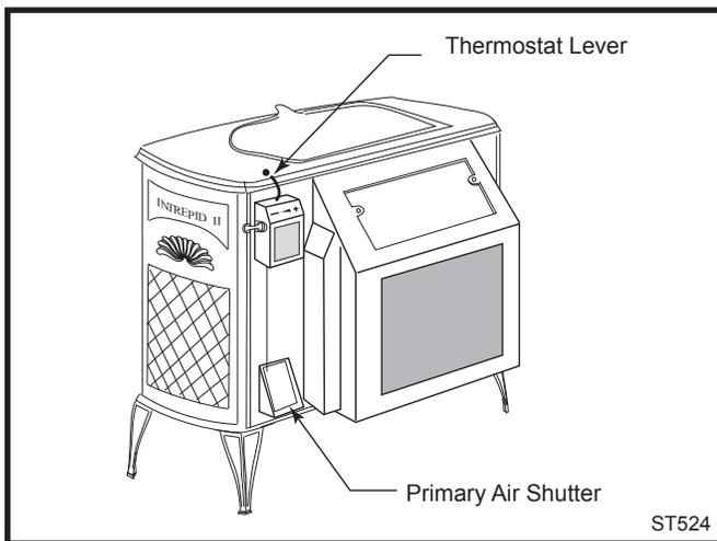
**Fig. 43** The primary air shutter must move freely.
