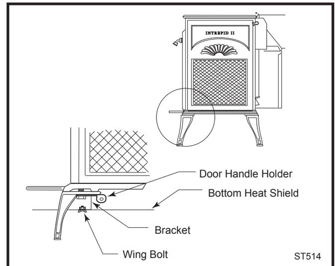
Fig. 29 Handle holder and heat shield positions.
