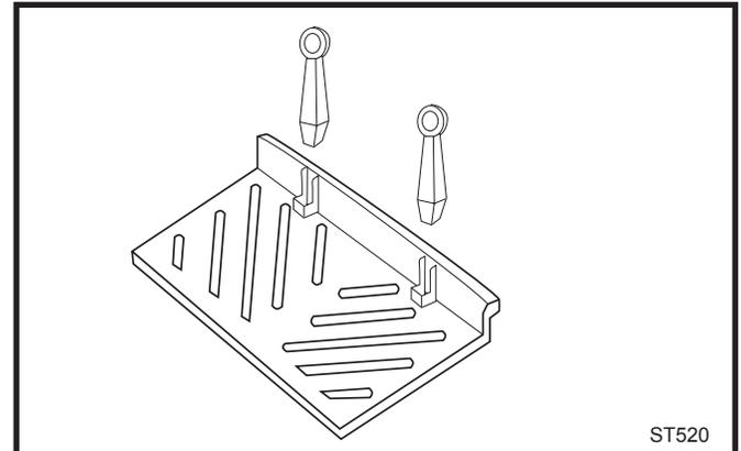
**Fig. 35** Remove the andirons for front loading.
