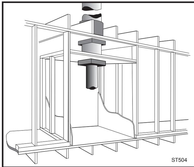
Fig. 18 Cutaway perspective of alcove installation.
