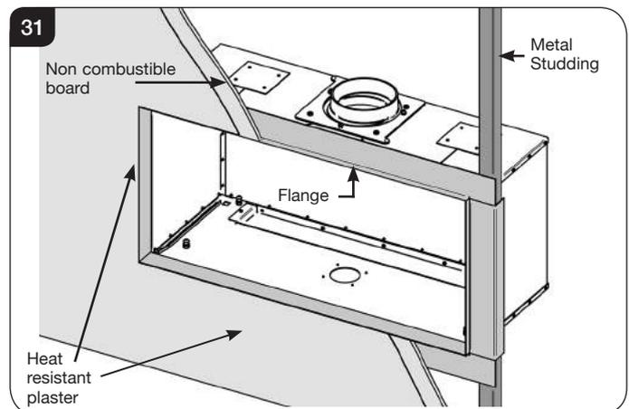
5.6 Fit plasterboard to the remaining chimney breast front.
