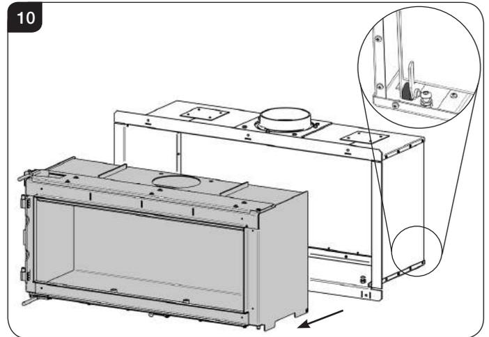
**Pull the inner box carefully forward to release from the cutouts. It should now slide smoothly out of the box. This will require at least two people.**
