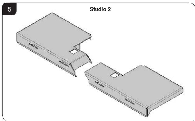
The Studio 2 baffle comes in two sections. To remove the baffle system first disengage the left hand side. The method of removal is the same for both sections.
