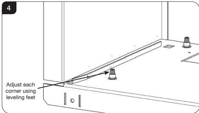
Wind the set screws down to the desired position in each corner.
