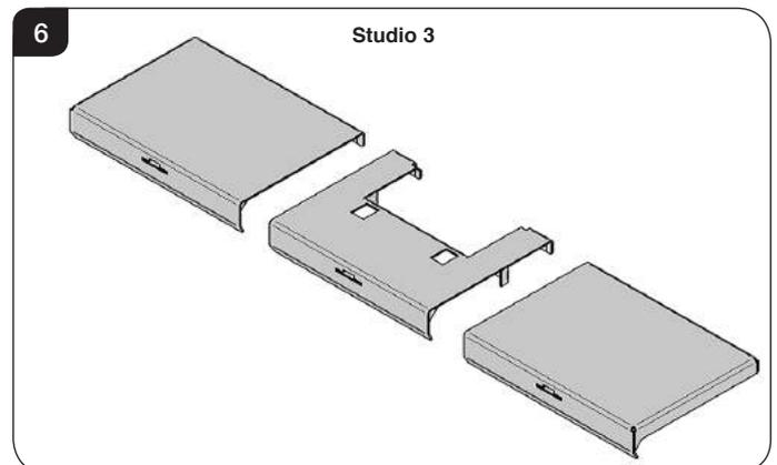
The Studio 3 baffle comes in three sections. To remove the baffle system the baffles must be taken out in the following order:
