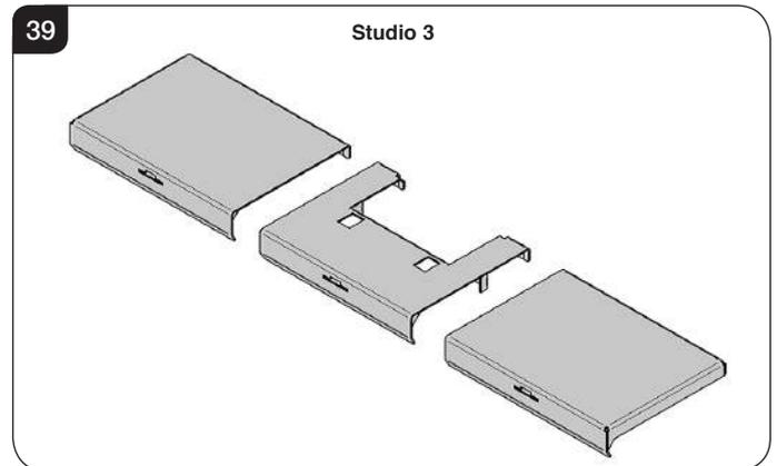
The Studio 3 baffle comes in three sections. To fit the baffle system the baffles must be placed in the firebox in the following order:
