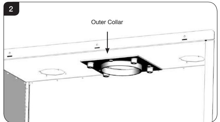
Using a 13 A/F Spanner remove the 3 bolts and remove outer collar.
