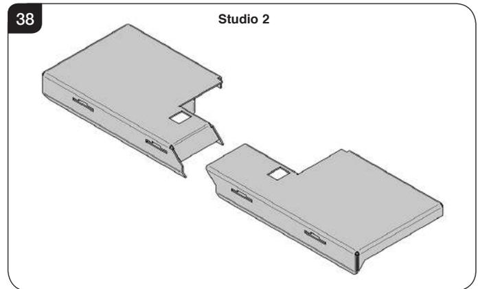
The Studio 2 baffle comes in two sections. Fit the right hand side baffle first. The method is the same for both sections.
