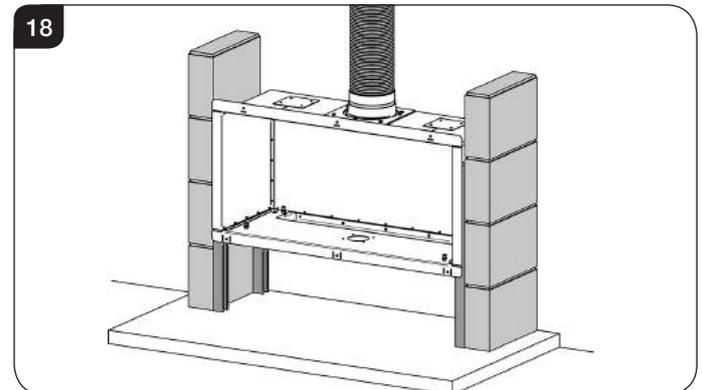
Ensure the clearances to combustibles are maintained, see Diagram 14.
