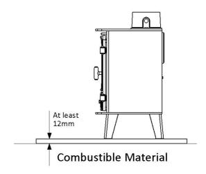
The hearth should extend at least 150 mm from the sides and rear of the stove, and at least 225 mm from the front of the stove.
