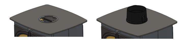
Place the Flue Gasket on the Top Plate Flue Exit. Place the Flue Collar on top of the Gasket. Secure to the four locating tabs, inside the flue outlet, using the M6 nuts & bolts supplied. Fit the 2 - M8 carriage bolts, washers & nuts into the Damper Holes, located on each side of the Flue Collar.
