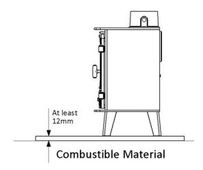
The hearth should extend at least 150 mm from the sides and rear of the stove, and at least 225 mm from the front of the stove.
