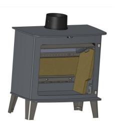
Slide the base of the Side Brick towards the centre of the stove and remove.
