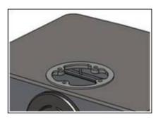
Place a flue outlet gasket in position on the top plate of the stove and lower the flue collar or blanking plate (as required) on to the stove top, taking care to line up the studs with the fixing holes.
