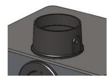
Place the Flue Gasket on the top, or rear outlet as required. Place the Flue Collar on top of the Gasket. Secure to the four locating tabs, inside the flue outlet, using the M6 screws supplied. Fit the 2 - M8 carriage bolts, washers & nuts into the Damper Holes, located on each side of the Flue Collar.
