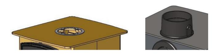
Place the Flue Gasket on the Top Plate Flue Exit. Place the Flue Collar on top of the Gasket. Secure to the four locating tabs, inside the flue outlet, using the M6 nuts & bolts supplied. Fit the 2 - M8 carriage bolts, washers & nuts into the Damper Holes, located on each side of the Flue Collar.
