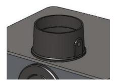
Place the Flue Gasket on the Top Plate Flue Exit. Place the Flue Collar on top of the Gasket. Secure to the four locating tabs, inside the flue outlet, using the M6 nuts & bolts supplied. Fit the 2 - M8 carriage bolts, washers & nuts into the Damper Holes, located on each side of the Flue Collar.
