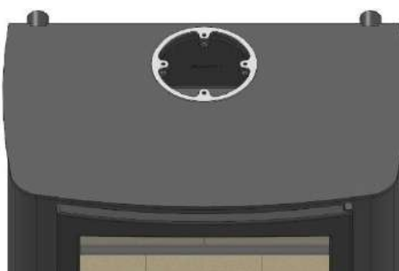
Place the flue collar gasket on the outlet to be used
