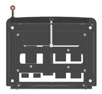
A) When the air control rod is pushed in fully then both the Primary and Secondary air intakes are in the closed position.
