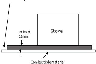
If the stove is not to stand in a recess, it may stand wholly above a hearth made of non-combustible board / sheet material or tiles, at least 12mm thick. The hearth should extend at least 150 mm from the sides and rear of the stove, and at least 300 mm from the front of the stove (350mm recommended).
