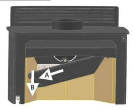
Push up and (A) drop one edge downward into the bottom of the stove and pull outwards (B).
