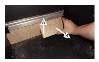
Push the brick upwards (A). Then pull the bottom edge of the rear brick forward and lift the brick out of the stove.
