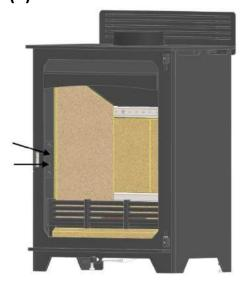
The door catch assembly is adjustable by loosening the four screws on the body of the stove. Diagram A shows the two outer screws which allows you to move the assembly up and down. Diagram B shows the two inner screws which allows you to move the assembly forward and backwards.
