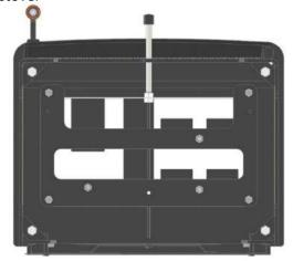
C) The air intake needs to be between 25% - 50% open to obtain the best result for burning wood.
