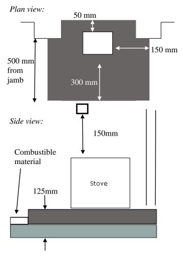
The stove can be recessed in a suitable sized fireplace but a permanent free air gap of at least 150mm on top and 50mm (although we recommend 150mm) around the sides and 50mm at the back of the stove to obtain maximum heat output and for access to the rear of the stove.
