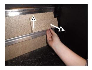
Push the brick upwards (A). Then pull the bottom edge of the rear brick forward (B) and lift the brick out of the stove.
