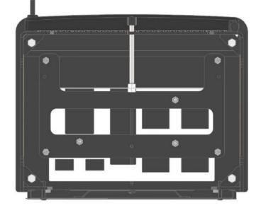
B) To operate pull the air control rod away from the stove. For the air control to be in the fully open position both Primary and Secondary pull the air control rod away from the stove until it stops. This is necessary for lighting the stove.
