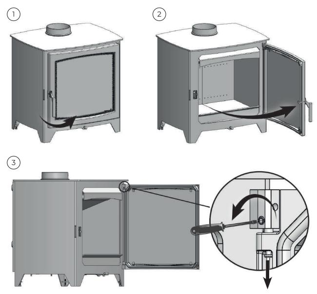
Loosen the grub screw as shown above in image 3. This will allow the hinge pin to drop down. Do this for both the top and lower hinge. Ensure the door is supported at all times.
