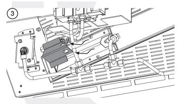
Replace with the correct size plate and secure the 2 nuts. Ensure that the lower edge of the plate is located over the venturi flange.
