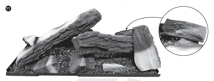
NOTE: ENSURE THAT THE LOGS ARE POSITIONED AS ABOVE. ONLY USE THE CORRECT AMOUNT OF LOGS AS SPECIFIED IN THE DIAGRAMS.
