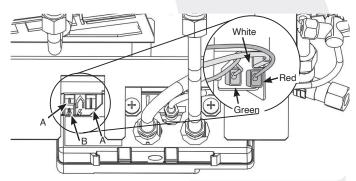
Replace with a new pilot assembly and check the spark gap.
