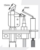
NOTE: Ensure the correct orientation when replacing.
