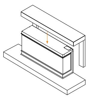
**17)** Carefully, lower the top section of the surround onto the top of the firebox.
