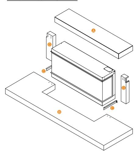
Before Installing the appliance onto the wall with the surround, secure the side trims each side of the appliance as shown below.
