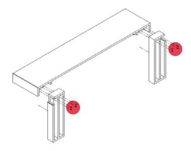
**16)** Screw the two legs of the surround from the rear onto the back of the top section of the surround as shown above
