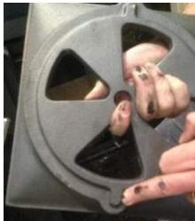
When re- installing base grate make sure lugs under the grate are in the quarter to three position and match the cutout in the base of the stove.
