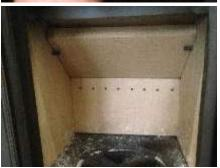
Remove lower baffle brick, slide baffle plate forward, then allow rear of baffle to drop down until baffle is vertical turn baffle and remove from chamber.
