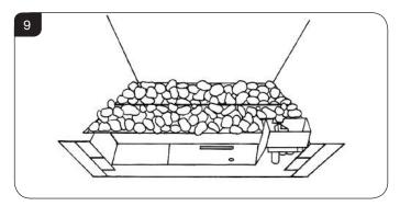
5.2 Lean the white stones against the burner ledges to disguise the ledges, see Diagram 10.
