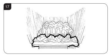
5.14 There are three sizes of coal used: 3 x Large, 4 x Small and 1 x Half Moon shaped. For identification, see Diagram 18.
