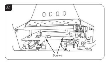
6.27 Undo 2 screws securing the gas valve to the bracket, see Diagram 33.
