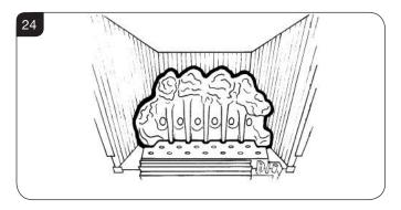
6.13 Place the front coal centrally in the channel at the front of the tray. The relationship between the front coal and the flame baffle is shown in Diagram 25.
