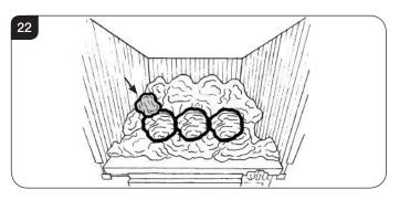
5.19 Place two of the remaining small coals in the spaces next to the first. The final small coal sits at the front right next to the large coals, see Diagram 23.
