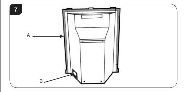
3.9 Gas pipe entry must come through the right-hand side of the box. The rubber seal must be cut using a sharp knife to allow the isolating elbow to pass through it. Ensure the rubber is not damaged when doing this, see Diagram 7, Arrow B.
