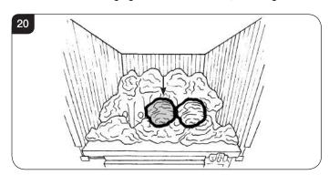
5.17 Place the third large coal next to the first middle coal and against the flame baffle, Diagram 21.
