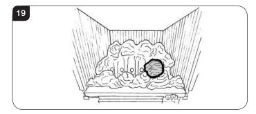
5.16 Place a second single large coal in the middle dent of the front coal resting against the flame baffle, see Diagram 20.
