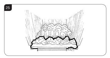
5.14 There are three sizes of coal used: 3 x Large, 4 x Small and 1 x Half Moon shaped. For identification, see Diagram 26.
