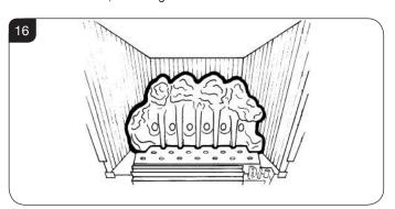
5.13 Place the front coal centrally in the channel at the front of the tray. The relationship between the front coal and the flame baffle is shown in Diagram 17.
