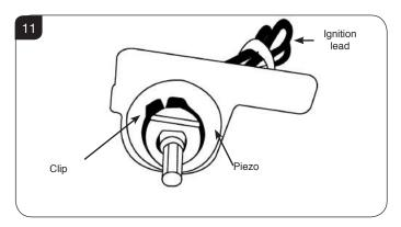
3.6 Rotate the Piezo anti-clockwise until the tab appears in the slot at the front, see Diagram 12.
