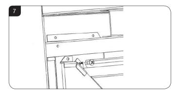
1.22 Carefully remove the enamel back panel by rotating it out of the firebox.
