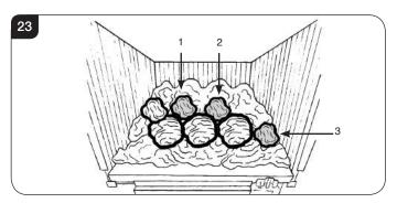
5.20 Finally position the Half Moon coal on the top right as shown, see Diagram 24.
