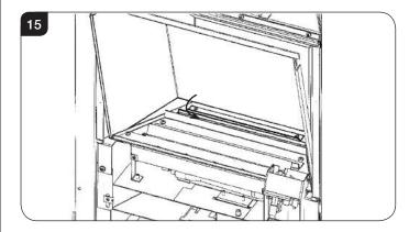
5.3 Secure the panel using the 2 upper brackets and the pozidriv screws, Diagram 16.
