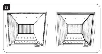
Locate the top panel on top of the sides and rear by lifting it up and forward inside the box.
