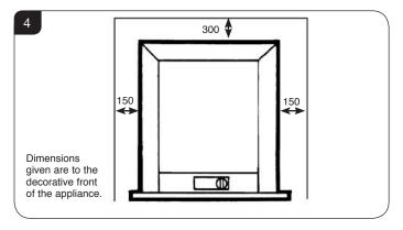
2.8 The maximum depth of combustible shelf is 150mm at a minimum height of 300mm above the decorative front.
