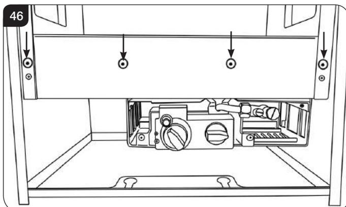
**!** UNDER NO CIRCUMSTANCES SHOULD THE APPLIANCE BE USED IF ANY OF THE GLASS FRAME RETAINING SCREWS ARE LOOSE OR MISSING.
