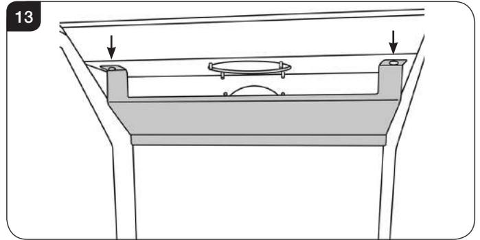
Note: When replacing the Rear Baffle ensure that the tab locates behind the rear panel slot, see Diagram 14.
