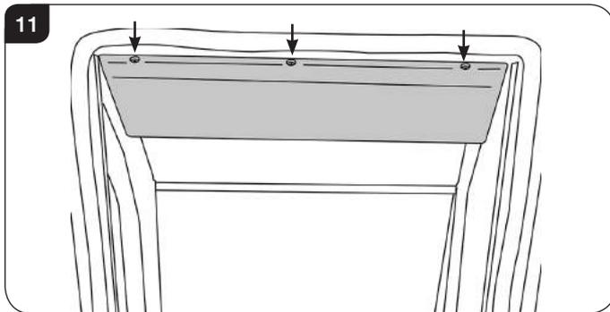
Note: when replacing the Main baffle ensure that the Main Baffle flap rests on the Rear Baffle, see Diagram 12.
