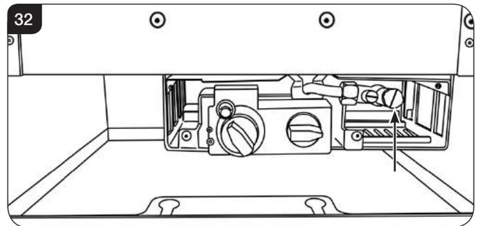
7.2 Connect a suitable pressure gauge to the test point located on the inlet fitting and turn the gas supply on. Light the appliance and check all gas joints for possible leaks. Turn the appliance to maximum and check that the supply pressure is as stated on the databadge. Turn the gas off and replace the test point screw, turn the gas on and check the test point for leaks.
