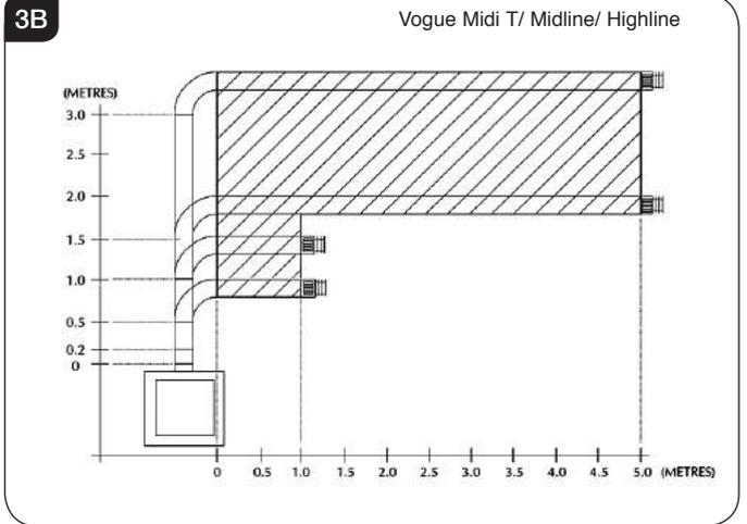
3.3 This kit provides the minimum materials. Extra lengths can be added to the vertical and horizontal sections; refer to Section 4.
