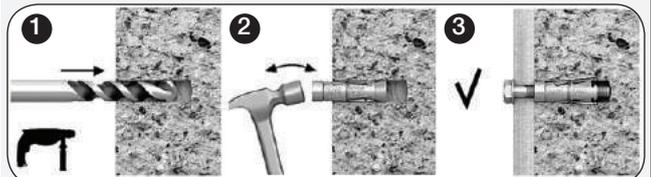
Ensure a minimum substrate thickness of 100mm.
