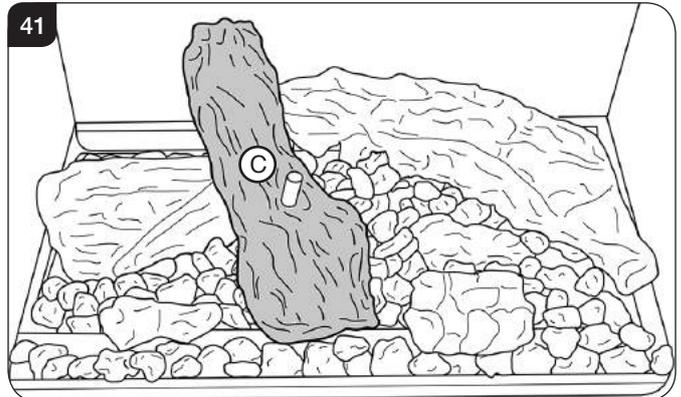
9.7 Log D fits onto the locating pin and rests on Log B, see Diagram 42.
