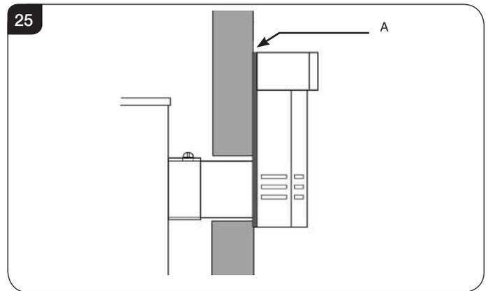
6.20 Feed the flue through the wall, making sure it runs smoothly.
