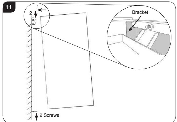
**NOTE:** The top rear edge of the appliance must locate between the back lip of the wall mounting bracket and the raised supports, see Diagram 12.
