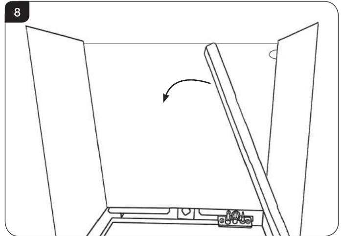
Support the rear panel when handling the last side and remove carefully.
