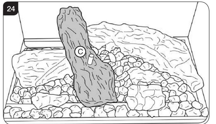
8.7 Log D fits onto the locating pin and rests on Log B, see Diagram 25.
