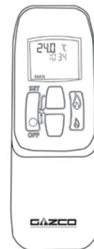
This remote controls the appliance from pilot ignition through to shut down.
