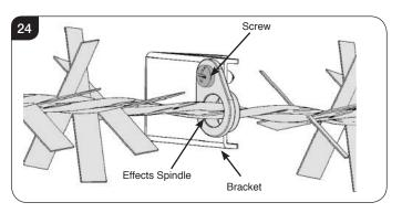
11.4 The Effects Spindle is attached to the Effects Motor by a rubber sleeve.
