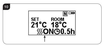
Note: It is normal for the fan heater to stop running for periods of time. This happens if the room temperature is higher than the temperature set on the control.
