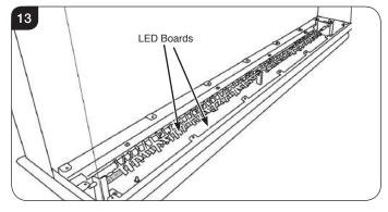
8.3 The LED boards are coupled together at the end of each board and held in place by clips, see Diagram 14.
