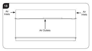
Dust build-up can inhibit efficient performance of the fan and lead to the safety cut-out operating.
