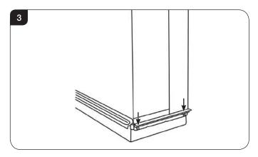
3.3 Fit the top Corner Side Glass Retainer bracket, ensuring all 3 screws are replaced, see Diagram 4.
