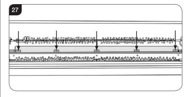
NOTE: When refitting the shield ensure that the lip curves down and towards the back. It will be necessary to lift the shield slightly to align the screws. Refit the screws from inside out.
