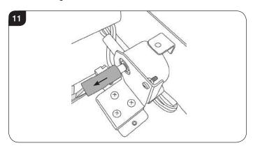
7.5 Withdraw the spindle from the left hand bracket, see Diagram 12.
