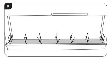
6.3 The flexible fuel bed can now be lifted out of the appliance.
