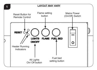
Note: The appliance will lose the memory for the light functions when the switch is set to the Off Position or the remote runs out of power.
