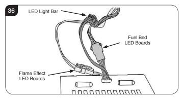
15.7 Replace in reverse order. Ensure all the leads are reconnected following the previous orientation.
