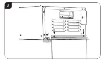
3.2 Remove the 2 Screws securing the lower bracket, see Diagram 3.
