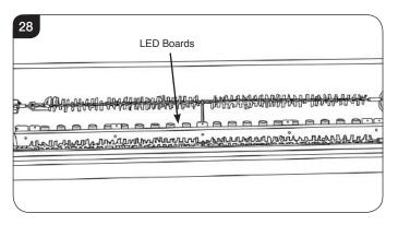
12.4 The LED boards are coupled together at the end of each board and held in place by clips, see Diagram 29.
