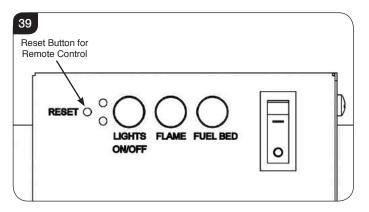
Resetting of the remote control is necessary if the appliance operates wrongly due to external interference signal and the remote control is not in use.
