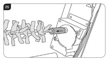
11.5 Withdraw the spindle from the left hand bracket, see Diagram 26.
