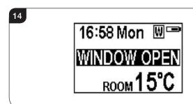
2b.45 After indoor temperature rise or manual intervention (by operating remote control), it will return to normal working state.
