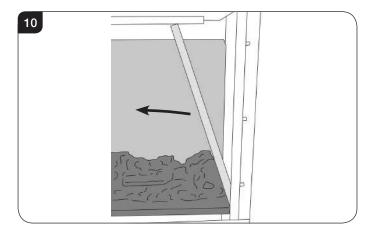
4.4 To remove the Left Hand liner first tilt inwards towards the centre of the firebox before lifting up and pulling out through the front of the firebox, see Diagram 10.
