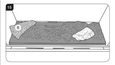
Place log A behind log B. The log will rest on the flat location plain shown in Diagram 13 with the right side against the right locating groove and the back against the rear liner, see Diagram 16.
