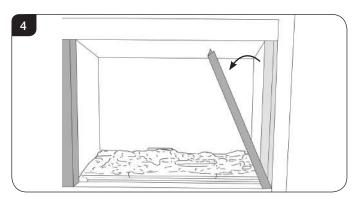
3.2 Lift out the bottom slotted trim, see Diagram 5.
