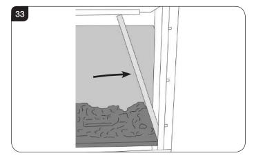
10.3 To fit the Left Hand liner insert through the front of the appliance tilting the top inwards towards the centre of the firebox before lowering into position, see Diagram 33.
