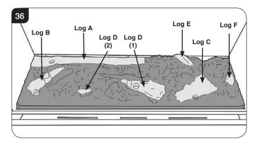
11.4 Place log C on the right hand side of the burner, see Diagram 37. The log will rest on the flat location point shown in Diagram 36.
