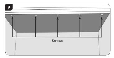
4.2 The baffle can now be removed by lowering the front edge and pulling forward through the front of the appliance. TAKE CARE NOT TO DAMAGE THE SIDE PANELS
