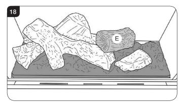
5.9 Position the right hand end of log F on the location point on the burner, see Diagram 13. Rest the left hand end of the log across the back end of log E, see Diagram 19. The back edge of log F should rest against the back liner.
