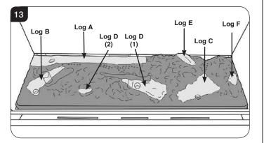
5.4 Place log C on the right hand side of the burner, see Diagram 13. The log will rest on the flat location point shown in Diagram 14.
