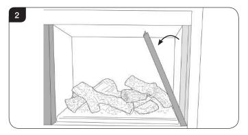
3.3 Lift out the bottom slotted trim, see Diagram 3.
