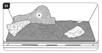
11.7 Position the right hand end of log D on the flat location plain on the burner, as shown in Diagram 36, Log D (1). Rest the left hand end of the log across log B, see Diagram 40. Ensure that the front branch rests in the location point on the burner, as shown in Diagram 36, Log D (2).
