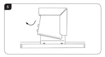
3.6 Remove the cover by sliding off in the direction of the arrow as shown in Diagram 6.
