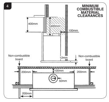
It is recommended that a marble slip or similar material is used when fitting cassette fireplaces into a plastered surface, in order to allow for heat dissipation. Also allow adequate time for newly plastered areas to dry out. Rapid drying can create cracks. If in doubt, seek the advice of a professional plasterer.
