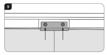
Remove the 2 screws to release the bracket and the liners, see Diagram 9.
