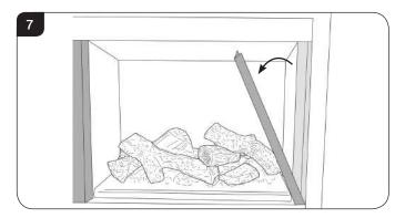
4.3 Lift out the bottom slotted trim, see Diagram 8.
