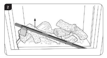
2.4 Disconnect the battery lead from the Battery Pack attached to the lower slotted trim, see Diagram 3.
