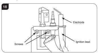
IMPORTANT The Ignition Lead and the Thermocouple need to be removed at the same time regardless of which needs to be replaced.
