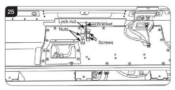
11.3 Remove the 2 screws and the bracket.
