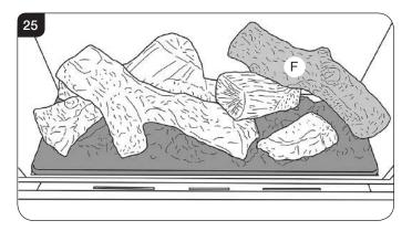
6.10 Separate the Embaglow material into smaller pieces and pull into shape to create a fine layer. 6.11 Place the pieces of Embaglow between the logs in the highlighted areas shown in Diagram 26. Ensure the material is placed loosely between the logs to create a random glow.
