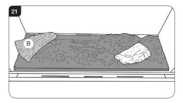
Place log A behind log B. The log will rest on the flat location plain shown in Diagram 19 with the left side against the left liner and the back against the rear liner, see Diagram 22.
