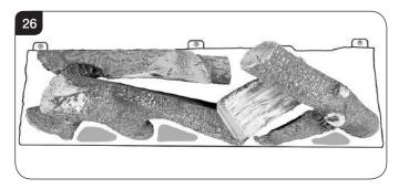
6.12 Once the fuel bed arrangement is complete, replace the glass frame and secure, see Section 4.
