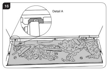
6.3 Slide the burner unit to the right, pull slightly forward and lift from the back. Carefully remove through the front of the appliance. Place carefully to one side.
