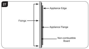
8a.10 Fit non-combustible board to the board around the appliance, see Diagram 28. Ensure distances to combustibles are observed, see Diagram 21.
