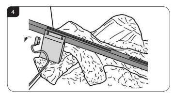
3.5 Remove the battery pack from the bracket, see Diagram 5.
