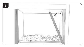
4.2 Lift out the bottom slotted trim, see Diagram 6. Note the orientation of the metal shield for reassembly.
