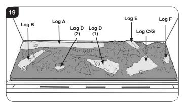
6.4 Place log C (Nat Gas) or G (LPG) on the right hand side of the burner, see Diagram 20. The log will rest on the flat location point shown in Diagram 19.
