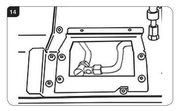
5.7 Remove the 15 screws securing the control assembly, see Diagram 15.
