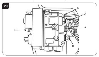
8.8 Remove the 2 screws securing the valve to the support bracket and withdraw the valve.
