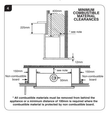
It is recommended that a marble slip or similar material is used when fitting cassette fireplaces into a plastered surface, in order to allow for heat dissipation. Also allow adequate time for newly plastered areas to dry out. Rapid drying can create cracks. If in doubt, seek the advice of a professional plasterer.
