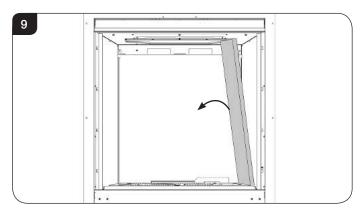
4.7 To remove the Left Hand liner first tilt inwards towards the centre of the firebox before lifting up and pulling out through the front of the firebox, see Diagram 9.
