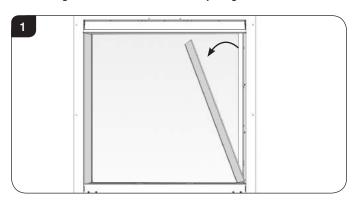
2.2 Lift out the bottom slotted trim, see Diagram 2.
