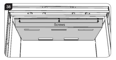
11.4 The baffle can now be removed by lowering the front edge and pulling forward through the front of the appliance.
