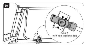
7.3 PURGE THE SUPPLY PIPE. This is essential to expel any debris that may block the gas controls.
