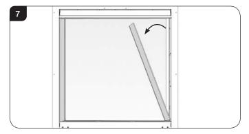
4.4 Lift out the bottom slotted trim, see Diagram 8.
