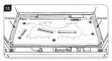
5.6 Remove the 4 screws from the corners of the burner unit, see Diagram 14.
