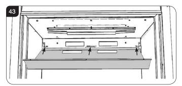
11.12 Replace the 3 screws to secure it to the roof of the firebox, See Diagram 44.
