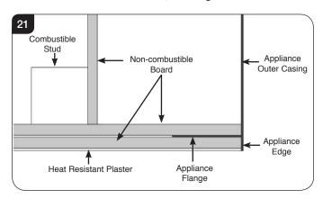
NOTE: If metal studwork is used, there is no need to fit non-combustible board to the inner face of the construction, see Diagram 22.
