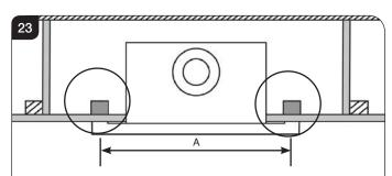
This diagram shows the minimum clearance position when installing the appliance into studwork - it is vital to ensure the batterning is wide enough to accommodate the fixings for the front.
