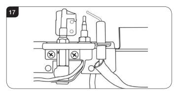
6.2 When replacing the pilot ensure the thermocouple follows its original route, i.e. along the pilot pipe. Attach the thermocouple to the pipe with new cable ties. 6.3 Set the spark gap, see Diagram 18.
