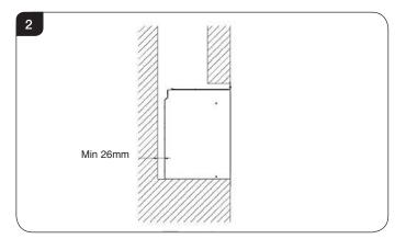
5.5 This appliance is not suitable for installation onto a combustible wall; all combustible materials must be removed from the area shown in Diagrams 3.
