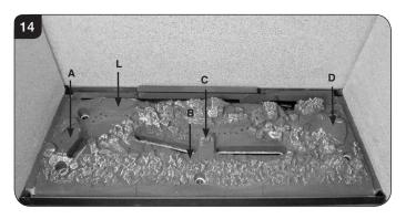
5.4 Place Log C on the stud in the centre of the burner, see Diagrams 14 & 15.
