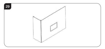
6.7 A removable access hatch must be left in the side of the chimney breast for future servicing and inspection of the appliance.
