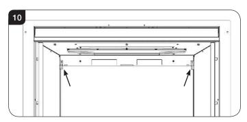
4.9 Remove the back liner by carefully lifting over the bottom bracket and twisting slightly to allow it to be removed through the front of the appliance, see Diagram 11.
