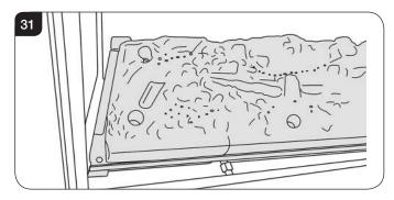
8.2 Slide the left hand side forward ensuring the burner tray and splitter plate fits around the mounting bracket, see Diagram 32.
