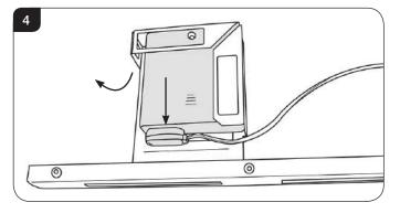
3.5 Remove the cover by sliding off in the direction of the arrow as shown in Diagram 5.
