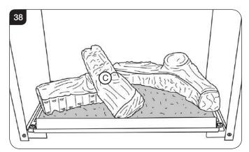
9.6 Log D fits onto the locating pin and rests on Log B, see Diagram 39.
