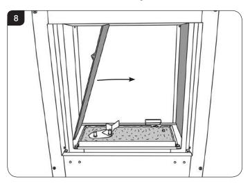
3.6 To remove the Left Hand liner first tilt inwards towards the centre of the firebox before lifting up and pulling out through the front of the firebox, see Diagram 9.
