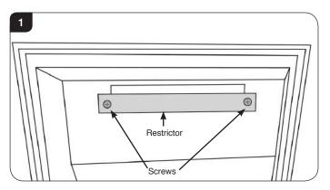
This is fitted from outside the appliance across the outlet at the top of the box with 2 screws provided.
