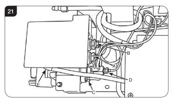
8.7 Remove the 2 screws securing the valve from the underside of the Control Assembly and withdraw the valve, see Diagram 22.
