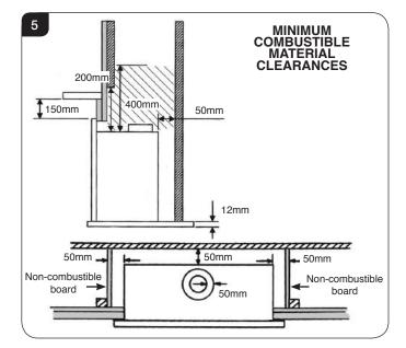
It is recommended that a marble slip or similar material is used when fitting cassette fireplaces into a plastered surface, in order to allow for heat dissipation. Also allow adequate time for newly plastered areas to dry out. Rapid drying can create cracks. If in doubt, seek the advice of a professional plasterer.
