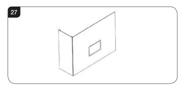
5.7 A removable access hatch must be left in the side of the chimney breast for future servicing and inspection of the appliance.
