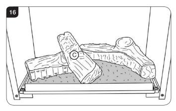
6.6 Log D fits onto the locating pin and rests on Log B, see Diagram 17.
