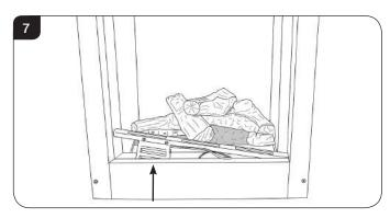
4.4 Disconnect the battery lead from the battery pack attached to the lower slotted trim and remove, see Diagram 8.
