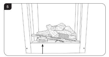
3.3 Disconnect the battery lead from the battery pack attached to the lower slotted trim and remove, see Diagram 6.
