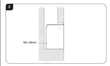
5.5 This appliance is not suitable for installation onto a combustible wall; all combustible materials must be removed from the area shown in Diagrams 4.
