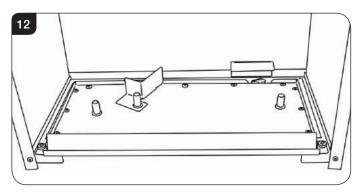
6.2 Place Log A in position on the 2 locating pins, see Diagram 13.
