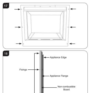
5a.10 Fit non-combustible board to the board around the appliance, see Diagram 19. Ensure distances to combustibles are observed, see Diagram 13.
