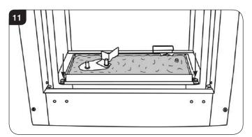
4.5 Remove the 2 screws at the front of the burner tray, see Diagram 12. TAKE CARE NOT TO DAMAGE THE FUELBED WHEN REMOVING THE SCREWS.
