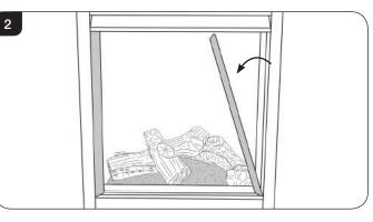
3.3 Lift out the bottom slotted trim, see Diagram 3. Note the orientation of the metal shield for reassembly.
