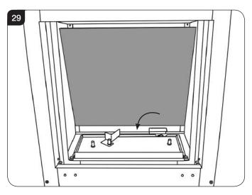
Support the rear liner until the side panels are in place.
