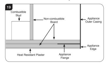
NOTE: If metal studwork is used, there is no need to fit non-combustible board to the face of the construction, see Diagram 20.
