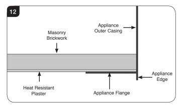
4b.6 The subframe for the decorative front can now be fitted by following the instructions supplied with the Front. NOTE: THE SUBFRAME MUST SIT FLUSH TO THE WALL LEVEL WITH THE APPLIANCE FLANGE.
