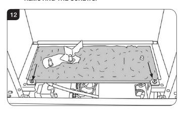
Note: At the same time as removing of the Main Burner the battery supply cable must be carefully disconnected from the control box.
