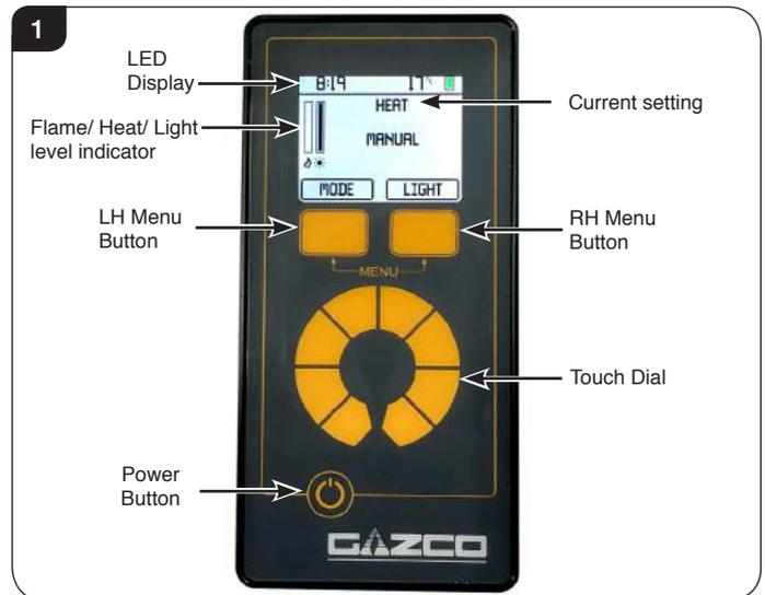
When carrying out any operations using the remote handset it is likely that it will go into Sleep Mode. Press the power button to reactivate.
