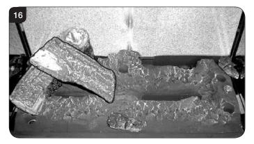
7.14 Place Log C on the right hand side of the burner. There is a hole on the underside of Log C which fits over the raised stud on the right of the burner. The back of the log should rest flush against the back panel, see Diagram 17.
