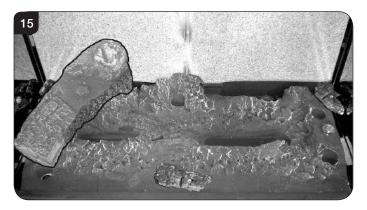
7.13 Place Log B on top of Log D. There is a hole on the underside of Log B which fits over the raised stud on Log D to secure in place. The right hand side of the log rests in the groove in the burner, see Diagram 16.
