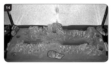
7.12 Place Log D on the left hand side of the burner. There is a hole on the underside of Log D which fits over the raised stud on the left of the burner. The back of the log should rest flat against the back panel, see Diagram 15.
