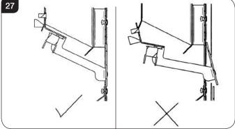
11.10 Replace the metal panel. There are spacers on the top edge to ensure the correct distance from the baffle. These interlock with the rear of the baffle, see Diagram 28.
