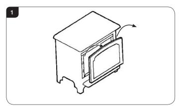
2.2 Remove the glass frame by undoing the fixing screws and lifting clear, see Diagram 2. Take care to support the glass window panel when removing the screws.
