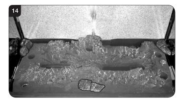
7.12 Place Log D on the left hand side of the burner. There is a hole on the underside of Log D which fits over the raised stud on the left of the burner. The back of the log should rest flat against the back panel, see Diagram 15.
