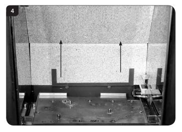
3.5 Slide the lower rear liner up and out of the lower bracket, see Diagram 5.
