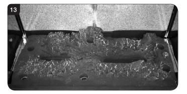
7.11 There are 3 embers. Place 2 embers in the back corners of the burner, resting in the cut outs, see Diagram 14. Place the last ember loosely at the front of the fuel bed to cover the hole in the centre.
