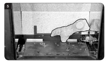
7.3 Place Log B over the two middle studs on the burner tray, see Diagram 6.
