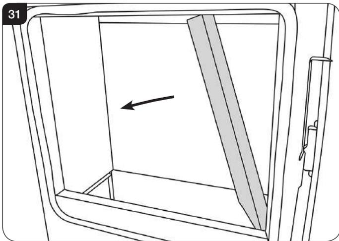
14.5 To remove the Left Hand liner first tilt inwards towards the centre of the firebox before lifting up and pulling out through the front of the firebox, see Diagram 31.
