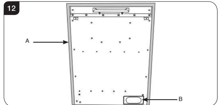
4a.12 Gas pipe entry must come through the rear of the box on the right-hand side. The rubber seal must be cut using a sharp knife to allow the isolating elbow to pass through it. Ensure the rubber is not damaged when doing this, see Diagram 12, Arrow B.
