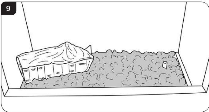
6.4 Log B is positioned on the right hand locating pin, and rests against the back liner, see Diagram 10.
