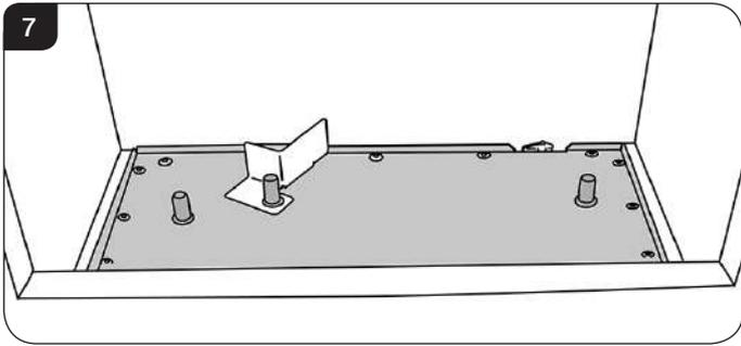
6.2 Place Log A in position on the 2 locating pins, see Diagram 8.
