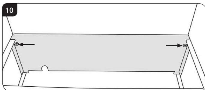
4a.10 Remove the 2 knockout holes on the rear of the box using a sharp hammer blow, see Diagram 11.
