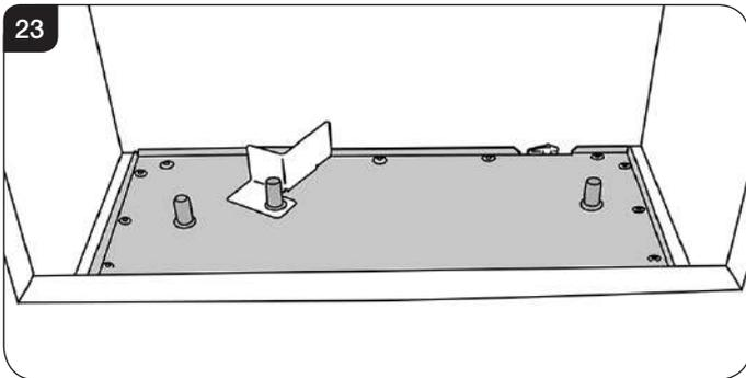
7.2 Place Log A in position on the 2 locating pins, see Diagram 24.
