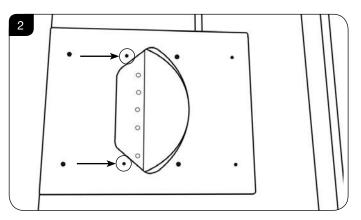
3.6 Position the flue spigot using the offset holes and the ones previously beneath the blanking plate. Secure the spigot and blanking plate in the new positions, see Diagram 3.
