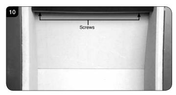
4.8 The baffle can now be removed through the front of the appliance.
