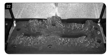
8.18 There are 3 embers. Place 2 embers in the back corners of the burner, resting in the cut outs, see Diagram 23. Place the last ember loosely at the front of the fuel bed to cover the hole in the centre.
