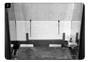
4.5 Slide the lower rear liner up and out of the lower bracket, see Diagram 8.
