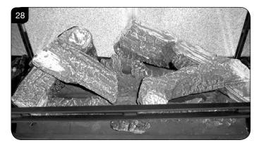
8.24 Once the logs are in place use some of the Embaglow wire wool provided and cover the ports in the burner tray with a liberal amount of fibres, in the highlighted areas shown in Diagram 29.
