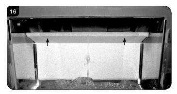
Once the baffles have been placed carefully to one side the liners can then been taken out in the following order.
