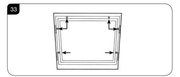
8.4 Ensure that the fibreglass seal on the back of the glass frame and replace the screws working from the top down. Tighten the screws evenly **DO NOT OVER TIGHTEN**, see Diagram 33.
