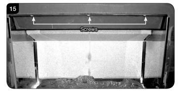
4.18 The baffle can now be removed through the front of the appliance.
