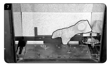
8.3 Place Log B over the two middle studs on the burner tray, see Diagram 8.
