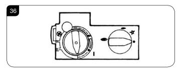
9.4 Press in the right-hand control knob and rotate anticlockwise until a click is heard. Continue to press in. The knob points to the pilot (\_\_).
