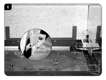
4.4 Gently lift the upper rear liner and pull forwards. With the panel raised it should be possible to remove from the liner brackets, see Diagram 7. Note: It may be necessary to use a flat object like a screwdriver to separate the two panels.
