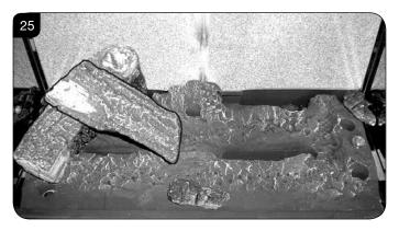
8.21 Place Log C on the right hand side of the burner. There is a hole on the underside of Log C which fits over the raised stud on the right of the burner. The back of the log should rest flush against the back panel, see Diagram 26.
