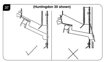
12.10 Replace the metal panel. There are spacers on the top edge to ensure the correct distance from the baffle. These interlock with the rear of the baffle, see Diagram 38.
