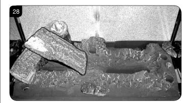
7.21 Place Log C on the right hand side of the burner. There is a hole on the underside of Log C which fits over the raised stud on the right of the burner. The back of the log should rest flush against the back panel, see Diagram 29.
