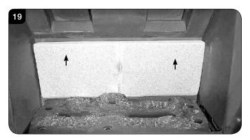
4.28 With the liners and baffle removed the firebox is clear for cleaning and maintenance, see Diagram 20.
