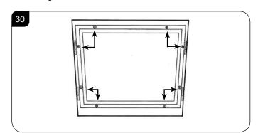
8.27 Replace ALL of the securing screws ensuring that a screw is present in all fixing slots.
