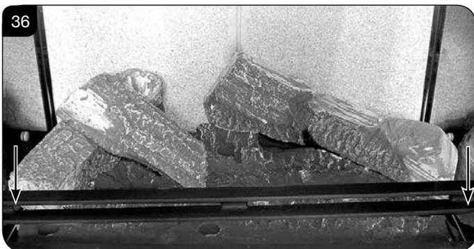
7.23 Place Log A across Log C. There is a hole on the underside of Log A which fits over the raised stud on Log C to secure in place. The small cut out on the left side of the log rests onto the log guard, see Diagram 37.
