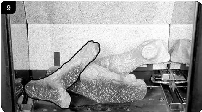
8.5 Place the small Ember at the front left of the firebox, against the rear of the log support bracket to obscure the reflection of the burner screw.
