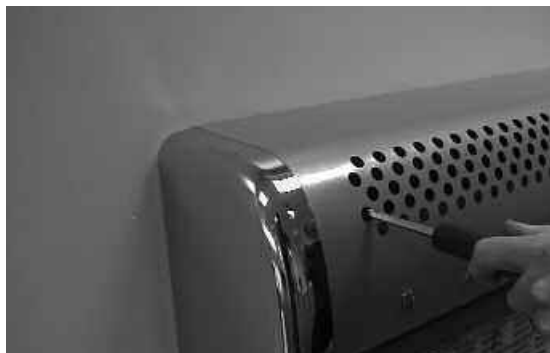
Fig. 10 Removing the Upper Outer Case Fixing Screws
