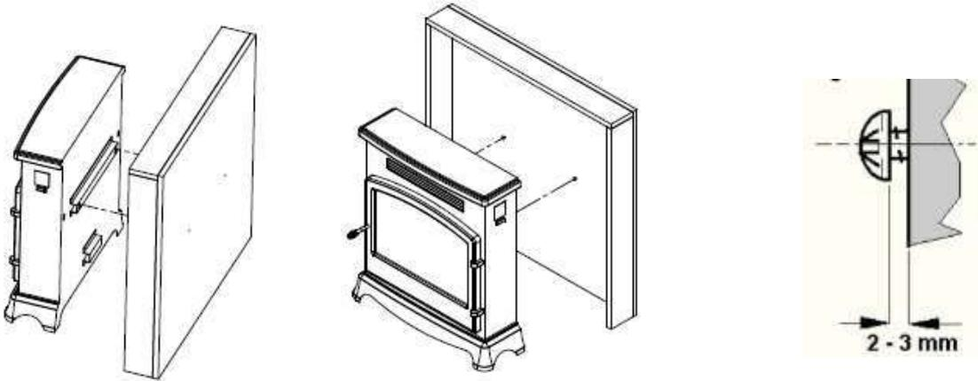
Should it be necessary to permanently fix the appliance into position, use the two brackets provided and fasten these to the underside of the top (Fig 7). Once these brackets have been fitted, offer the appliance to the wall and mark the fixing positions. Remove appliance and drill / plug wall with correct fixings for the medium. The stove can now be put back into position and screwed in place via the fixing brackets (Fig 8).
