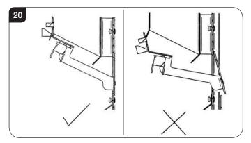
12.10 Replace the metal panel. There are spacers on the top edge to ensure the correct distance from the baffle. These interlock with the rear of the baffle, see Diagram 21.
