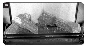
7.7 Place Log A across Log C. There is a hole on the underside of Log A which fits over the raised stud on Log C to secure in place. The small cut out on the left side of the log rests onto the log guard, see Diagram 11.
