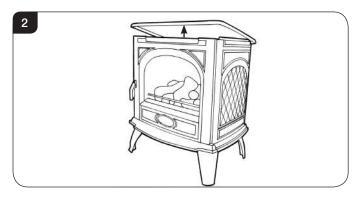
5.4 Lift the front upwards until it is clear of the slots and pull away from the appliance, see Diagram 3.
