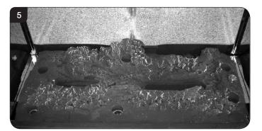
7.2 There are 3 embers. Place 2 embers in the back corners of the burner, resting in the cut outs, see Diagram 6. Place the last ember loosely at the front of the fuel bed to cover the hole in the centre.
