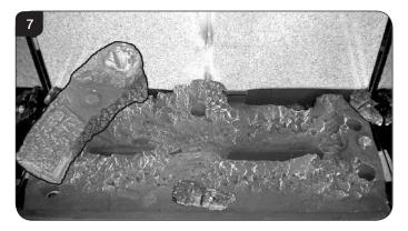
7.4 Place Log B on top of Log D. There is a hole on the underside of Log B which fits over the raised stud on Log D to secure in place. The right hand side of the log rests in the groove in the burner, see Diagram 8.
