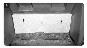
4.15 With the liners and baffle removed the firebox is clear for cleaning and maintenance, see Diagram 9.
