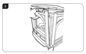
5.4 Remove the glass frame by undoing the fixing screws and lifting clear, see Diagram 4. Take care to support the glass window panel when removing the screws.
