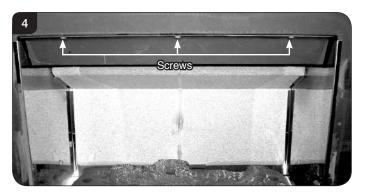
4.5 The baffle can now be removed through the front of the appliance.
