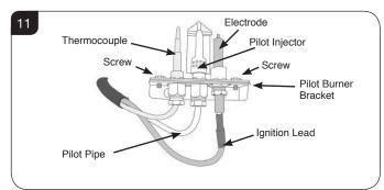
NOTE: Ensure the sealant surrounding the Electrode and Thermocouple leads is replaced if disturbed or removed whilst gaining access to these components.
