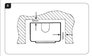
8.4 In a non-combustible recess be careful to allow enough clearance at the sides and rear of the appliance to perform spillage tests and reach the controls.
