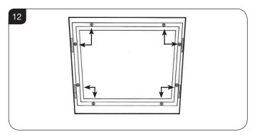
7.9 Replace ALL of the securing screws ensuring that a screw is present in all fixing slots.
