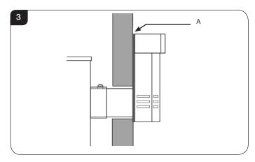
3.23 Feed the flue through the wall, making sure it runs smoothly.
