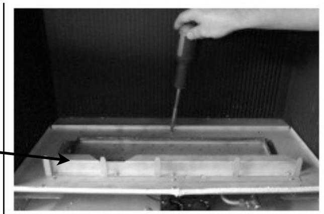
Whilst lifting the Assembly at the rear, rotate it towards you and remove it from the Fire taking care not to foul the Side Liners of the fire.
