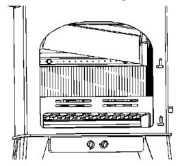
To install the Baffle, slide the left-hand end of the Baffle up, and over the support. Push the Baffle to the left until the right-hand edge clears the other support. Slide the Baffle back to the right until it sits centrally in the stove. Check that the two tabs at the front of the Baffle are between the Baffle Supports.
