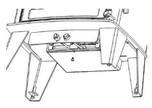
To remove the Air Valve Cassette, first adjust both control knobs to maximum open (turn fully clockwise). Then, undo the Air Valve Cassette retaining screw located under the Air Cassette housing, and remove it from the stove.
