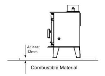
The hearth should extend at least 150 mm from the sides and rear of the stove, and at least 225 mm from the front of the stove.
