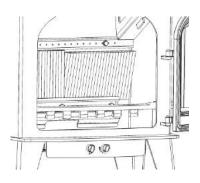
Pull the top edge of each Rear Brick forward and lift the brick out of the Stove.
