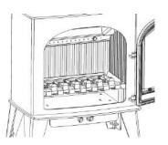
2. Remove all of the Grate Bars. Take care to notice which are the upper and which are the lower bars. This will allow correct replacement.
