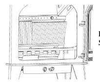
Pull the top edge of each Rear Brick forward and lift the brick out of the Stove.
