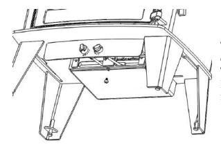
To remove the Air Valve Cassette, first adjust both control knobs to maximum open (turn fully clockwise). Then, undo the Air Valve Cassette retaining screw located under the Air Cassette housing, and remove it from the stove.
