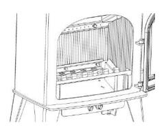
3. Slide the front edge of each Side Plate towards the centre of the stove. Lift the Side Plates and remove.
