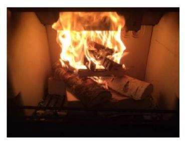
Light the firelighter(s), leaving the air controls fully open and close the door. It may not be necessary to leave the door open but DO NOT leave the stove unattended if you find it necessary to leave the door ajar.
