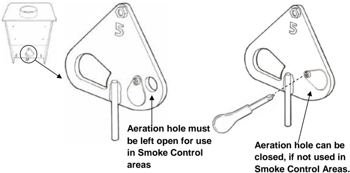
*This type of plate is only supplied with the 9103, 9104, 9105 & 9108 stoves which are approved for use in Smoke Control Areas. This type of plate is not supplied with the 9112 which is not approved.*
