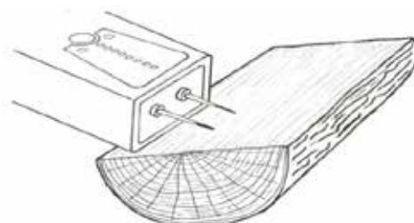
Simply putting the contact pins onto the surface will not give an accurate reading, as it may tell you that the surface is dry whilst the interior of the log may well be damp.
