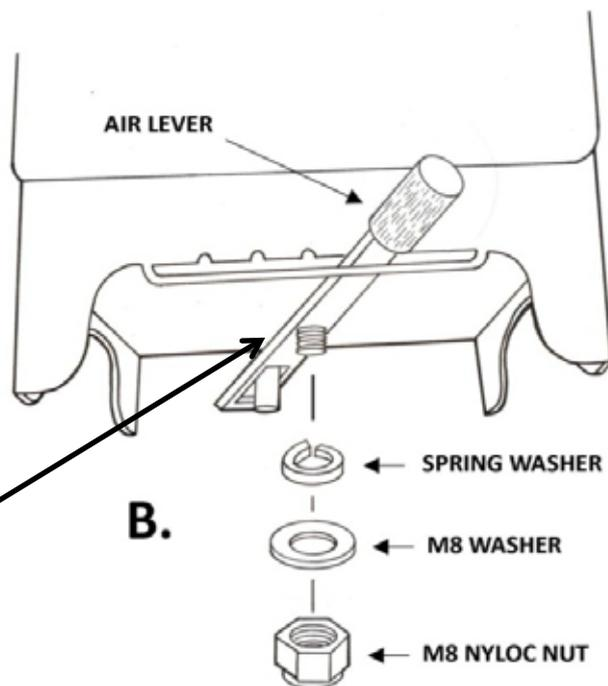
Put the M10 washer over the threaded stud, push the air lever through the slot in the front of the stove, locate the end of the lever over the air plate bar and threaded stud, ensuring that the M10 washer sits over the unthreaded shoulder of the stud. Assemble the remaining washers and nut as per diagram (B) using the 13mm spanner. Please ensure the lever moves from left to right with just a little resistance to ensure it stays in place.
