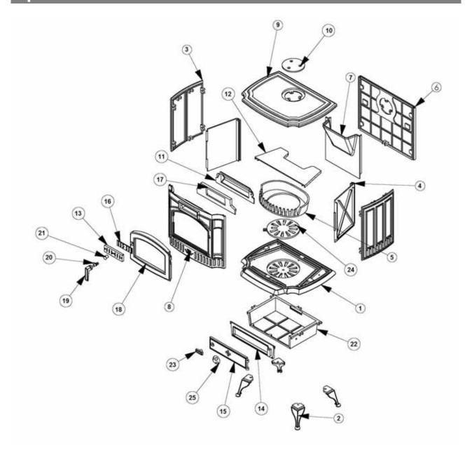
(1) Base Casting (2) Legs (3) Side Castings (4) Side Firebricks
