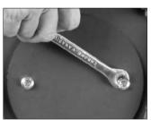
Remove the inner blanking plate by removing the two bolts
