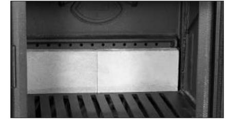
combustion chamber. Remove the second side brick in the same manner, the flue baffle can now be removed by lowering the front edge and rotating the baffle and removing through the front door.
